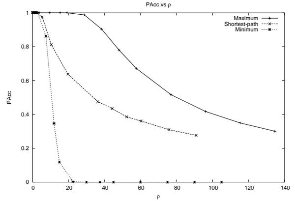
Figure 9: Call acceptance probability of single-hop calls using shortest-path routing vs varying load.
