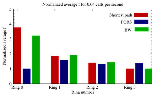
Figure 15: The normalized average fraction of calls being routed to a node with increasing distance from the center. The arrival rate is 0.04 calls per second at a node.
