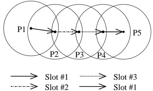
**Figure 6: Multi-hop call setup.**  $R(P_1)$  needs slot #1 to be free.  $R(P_2)$  now cannot use slot #1 and requires slot #2 (some other slot) to be free.  $R(P_3)$  cannot use slots #1 and #2, and requires slot #3 (any other slot) to be free.  $R(P_4)$  can transmit in slot #1 if it is free.
