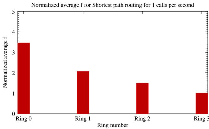
Figure 8: The normalized average fraction of calls being routed to a node with increasing distance from the center for shortest-path routing. The arrival rate is 1 calls per second at a node.
