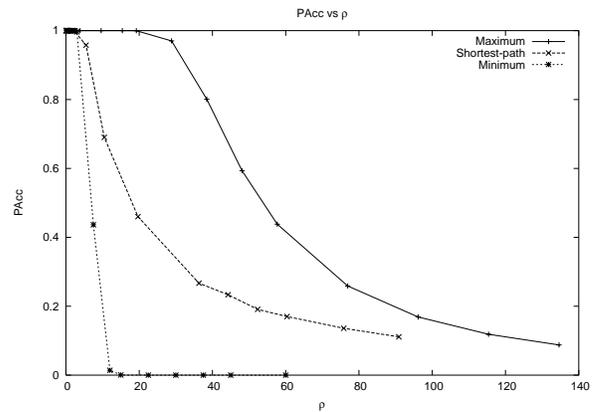
Figure 10: Call acceptance probability of 2-hop calls using shortest-path routing vs varying load.
