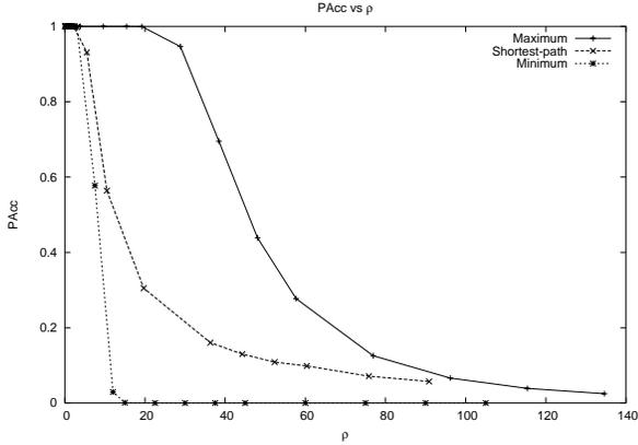
**Figure 11: Call acceptance probability of 3-hop calls using shortest-path routing vs varying load.**
