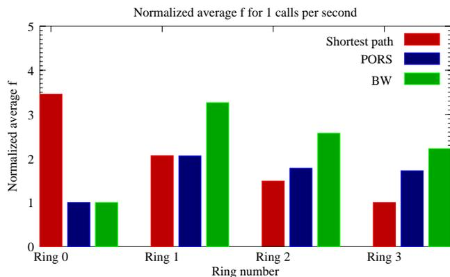
Figure 16: The normalized average fraction of calls being routed to a node with increasing distance from the center. The arrival rate is 1 calls per second at a node.
