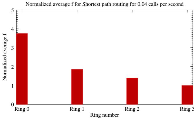
Figure 7: The normalized average fraction of calls being routed to a node with increasing distance from the center for shortest-path routing. The arrival rate is 0.04 calls per second at a node.
