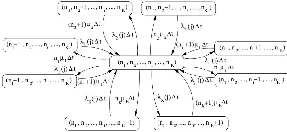
**Figure 4: The transitions into and out of one of the states of the Markov process representing the region  $R(j)$ . For the state  $(n_1, n_2, \dots, n_K)$ ,  $n_1 > 0, n_2 > 0, \dots, n_K > 0$ .**
