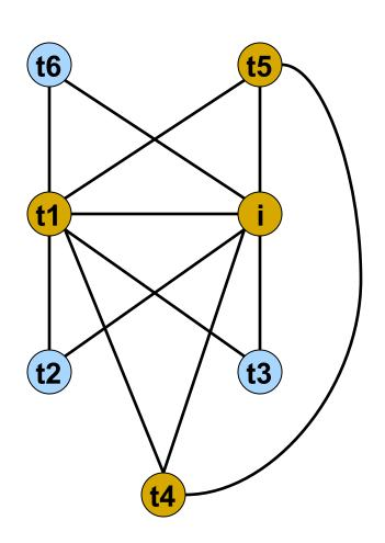
Assume 3 registers. Nodes t6,t2, and t3 are first pushed onto a stack during reduction.
