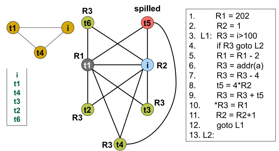
t5: spilled node, will be provided with a temporary register during code generation
