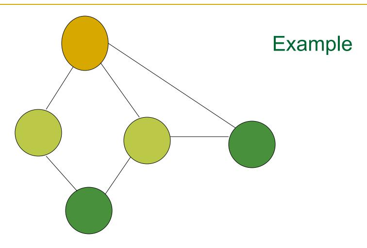
Here R = 3 and the graph is 3-colourable No spilling is necessary
