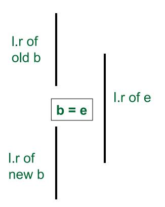
copy subsumption is not possible; lr(e) and lr(new b) interfere
