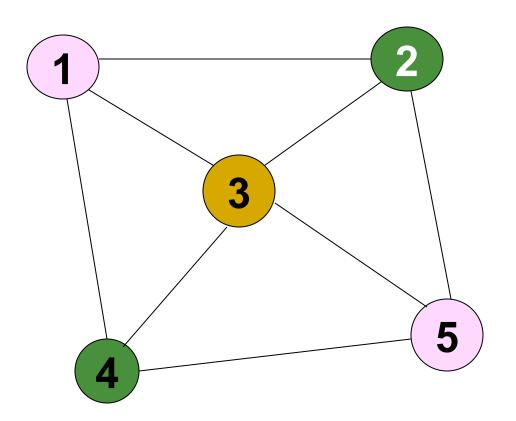
Say, 1 is chosen for spilling. Push it onto the stack, and remove it from the graph. The remaining graph (2,3,4,5) is 3-colourable. Now, when 1 is popped from the colouring stack, there is a colour with which 1 can be coloured. It need not be spilled.
