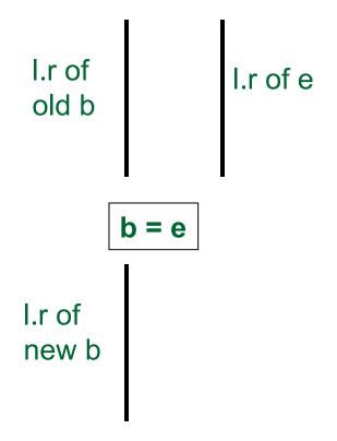
copy subsumption is possible; lr(e) and lr(new b) do not interfere
