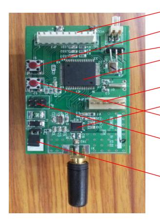
ADC/IO port User button UART Power jumper **Microcontroller**(ATMEGA1281V) UART port Transceiver(AT86RF230) Reset button **Programming port** Programming jumper
