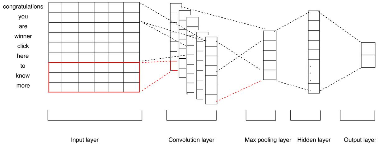
Fig. 1. CNN architecture for an example tweet.
