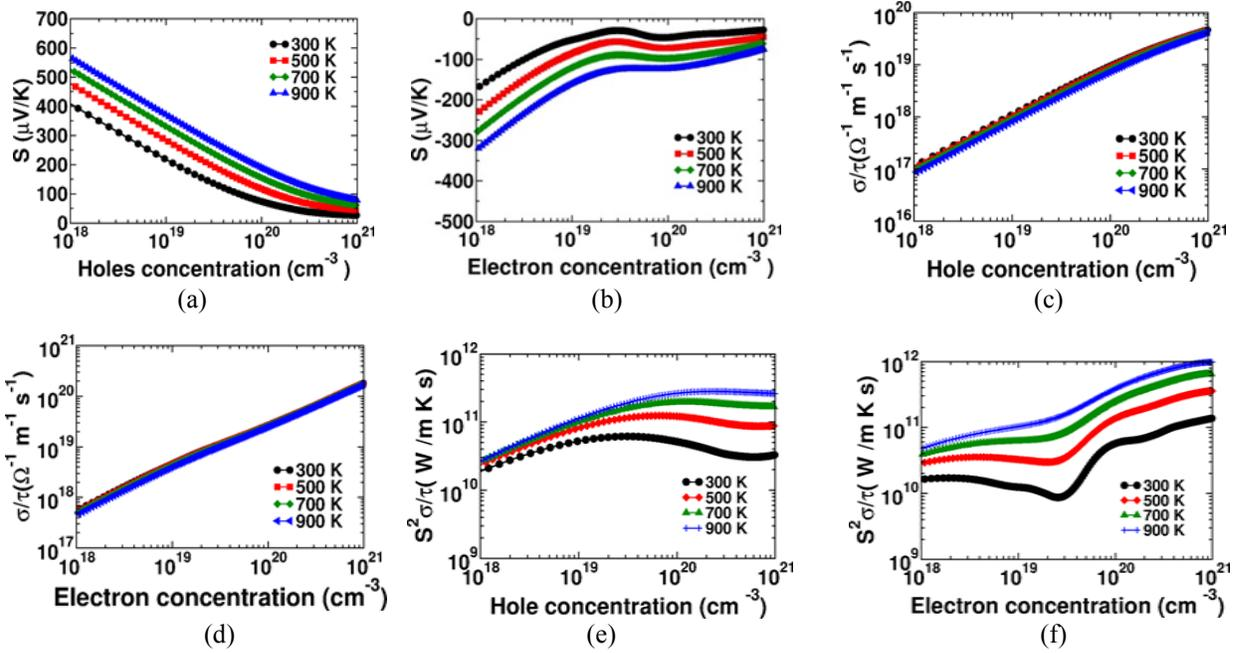
**FIGURE 2.** (a, b) Variation of thermopower, (c, d) electrical conductivity scaled by relaxation time and (e, f) power-factor with holes and electrons.
