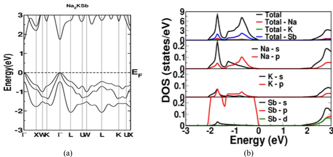
FIGURE 1. (a) Calculated band structure and (b) density of states of Na<sub>2</sub>KSb
