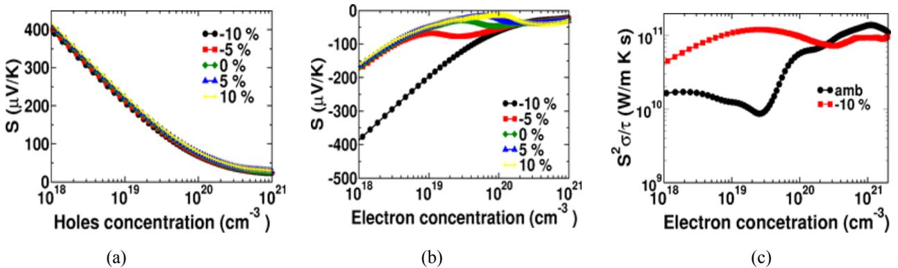
**FIGURE 3.** (a) thermopower for holes, (b) thermopower for electrons, (c) Power-factor for electron as a function of strain
