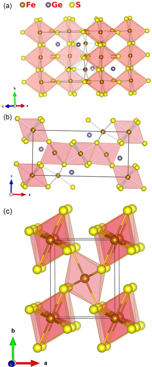
**Figure 1.** Crystal structure of (a) edge-sharing octahedra and (b) vertex-sharing octahedra of  $\text{Fe}_2\text{GeS}_4$  compared with (c) marcasite  $\text{FeS}_2$ .
