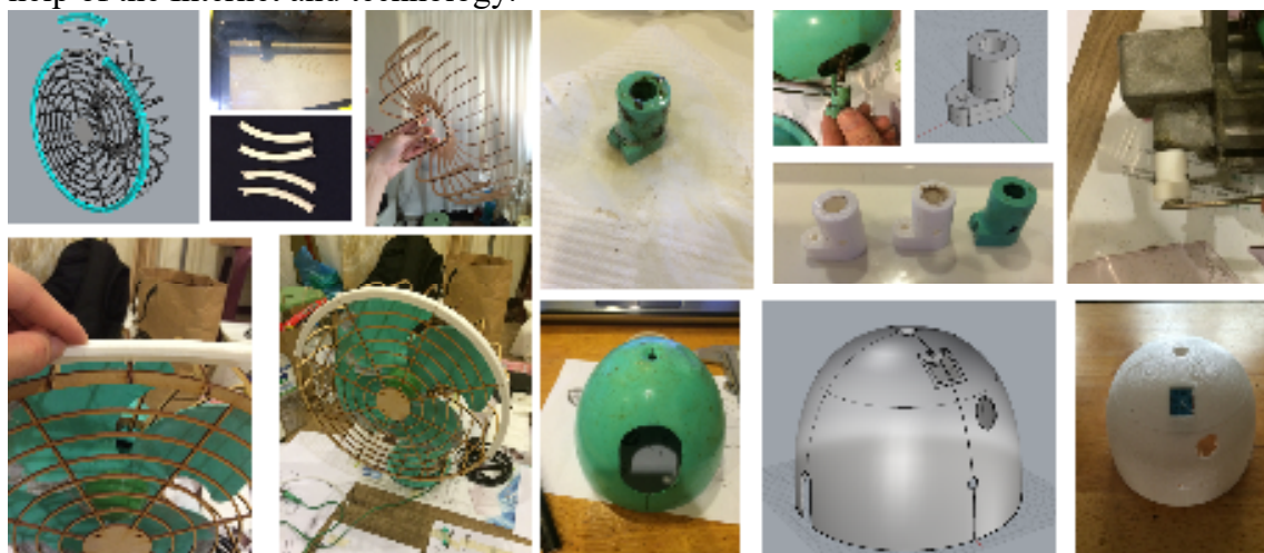
Fig. 1. Repairing process aided by digital fabrication techniques
