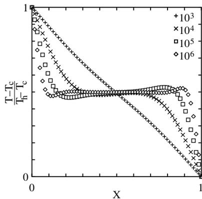
Fig. 5. Temperature profiles ( $y/H = 0.5$ ) for  $Ra = 10^3$  to  $Ra = 10^6$ .
