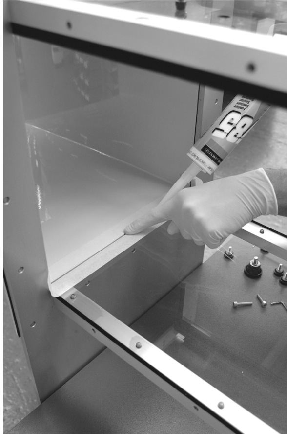
Figure 14 Apply Silicone to the Cone-Working Section Joint.
