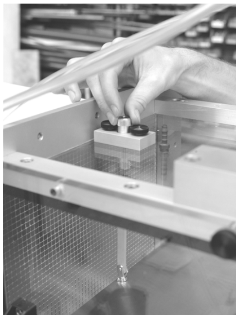
Figure 5 Fit the Adjuster Mounting in Place of the Rear Pitot Tube.
