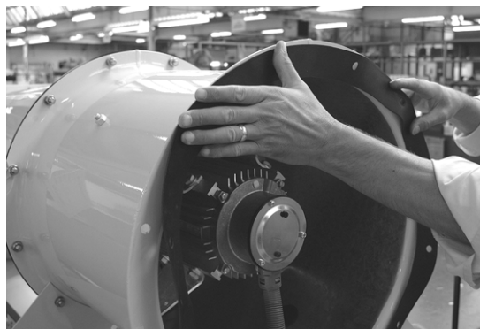
Figure 13 Make Sure the Round Black Gasket is In Place on the Fan Unit Flange
