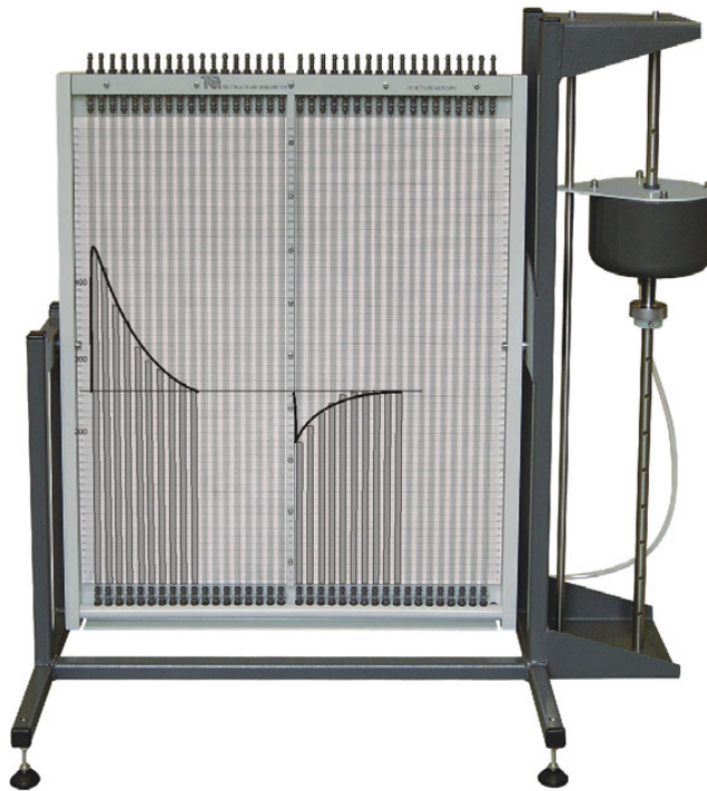
Figure 11 Example of Levels with Odd then Even Tapping Connections on the TecQuipment AFA1 Multi-tube Manometer
