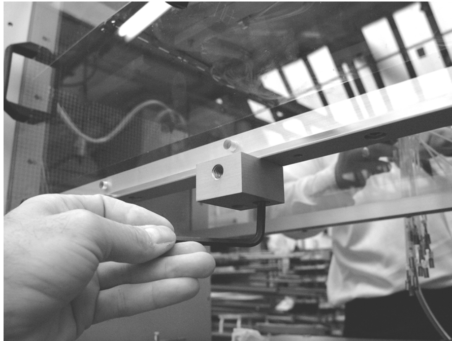
Figure 8 Make Sure Bottom Mounting is turned around so that the Hole is Visible
