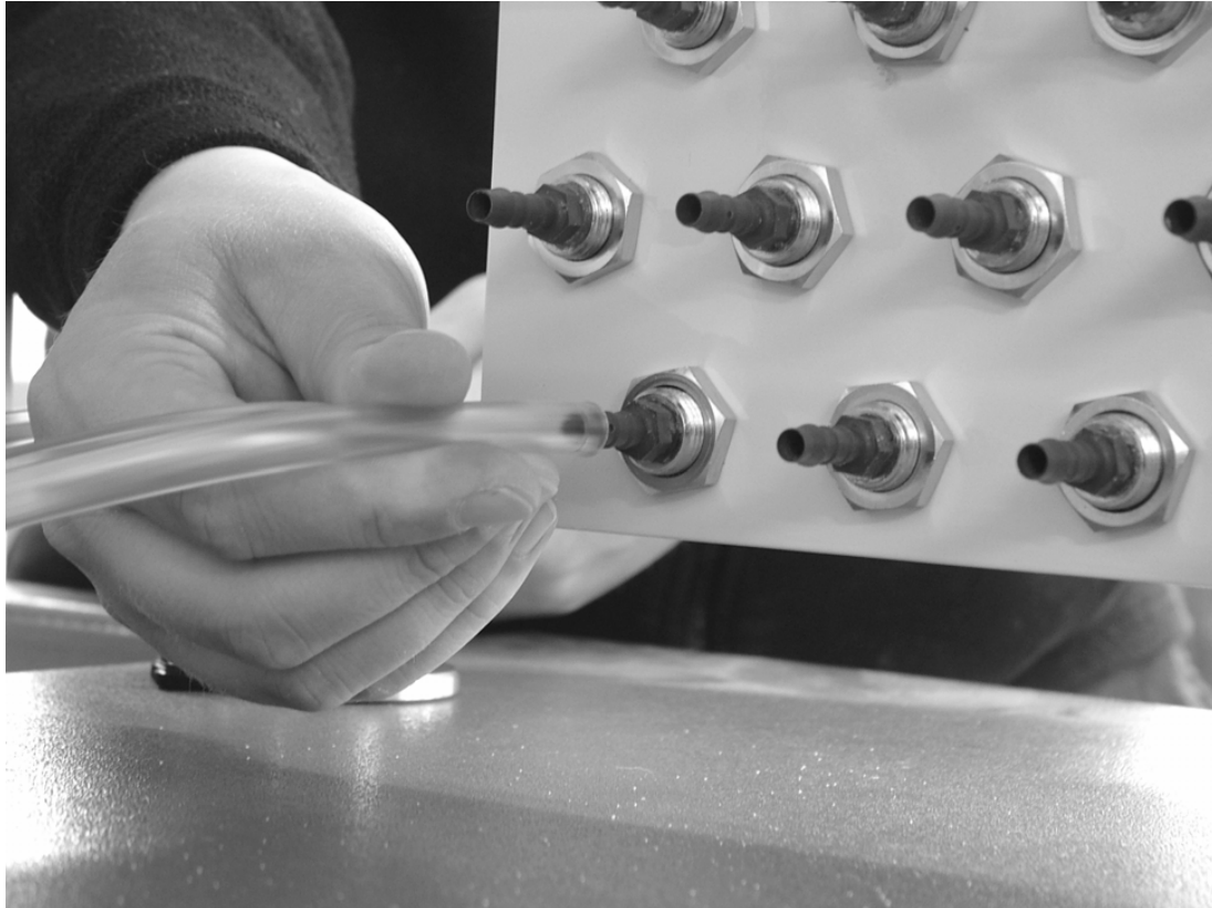
Figure 11 Use the Clear Pipe Supplied to Connect to the Back Sockets
