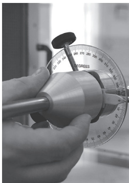
Figure 5 Slide Protractor onto Hollow Support Shaft and Set to Zero.
