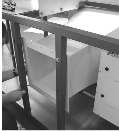
Figure 10 Unbolt the Effuser From Under the Main Frame
