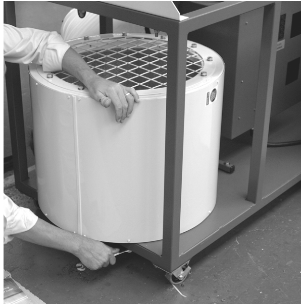
Figure 12 Unbolt Silencer from Frame
