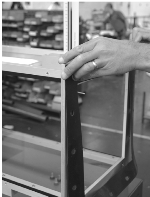
Figure 11 Hold the Square Gasket Against the Working Section
