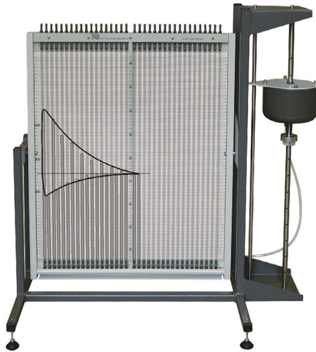
Figure 10 Example of Levels with Alternate Odd and Even Tapping Connections on the TecQuipment AFA1 Multi-tube Manometer
