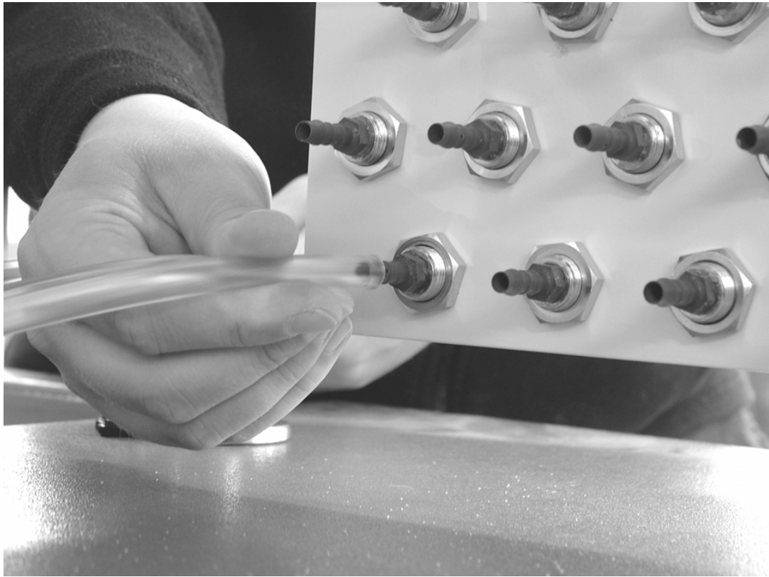
Figure 8 Use Pipe Supplied to Connect Back Connections to a Suitable Pressure Measurement Device
