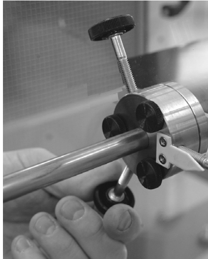
Figure 4 Tighten the Three Lock Screws of the Model Holder
