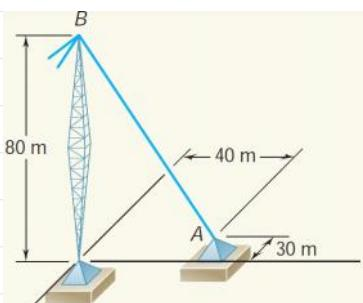
A tower guy wire is anchored by means of a bolt at A. The tension in the wire is 2500 N. Determine (a) the components  $F_x, F_y, F_z$  of the force acting on the bolt, (b) the angles  $\theta_x, \theta_y, \theta_z$  defining the direction of the force.
