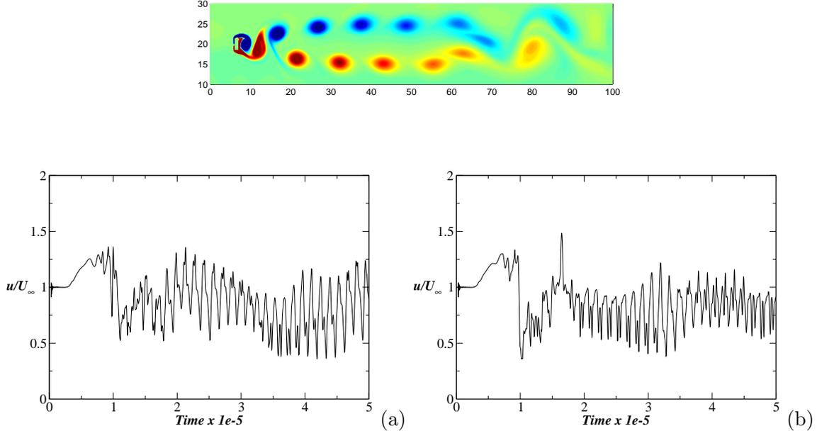
Figure 8: Time trace of total velocity downstream of the body for  $A = 3$ ,  $Fr = 5$  and  $Re = 200$  from locations 3 and 4. The  $St$  for (a) and (b) is equal 0.1050
