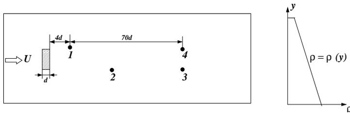
Figure 3: A schematic view of the computational domain showing four monitor points. The figure is not to scale.
