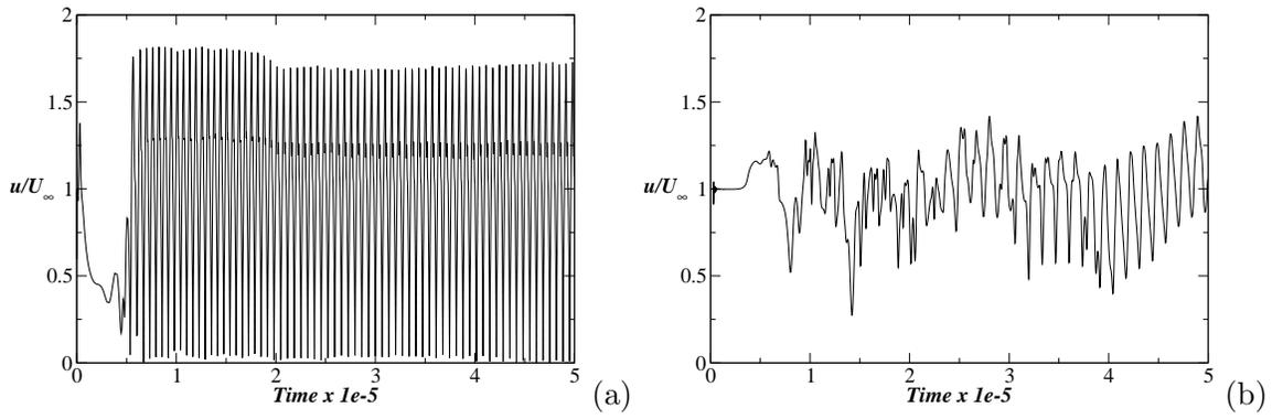
Figure 6: Time trace of total velocity downstream of the body for  $A = 3$ ,  $Fr = \infty$  and  $Re = 200$  from locations 1 and 4. The  $St$  for (a) is 0.222 and for (b) is 0.1125
