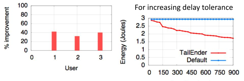
TailEnder nearly halves the energy consumption for a 15 minute delay tolerance. (Over GSM, improvement is only 25%)
