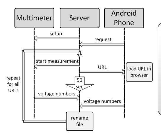
Server controls the phone and multimeter:
