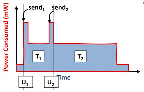
Last-Trigger-Policy: Assign asynchronous (tail) energy to the last active system call
