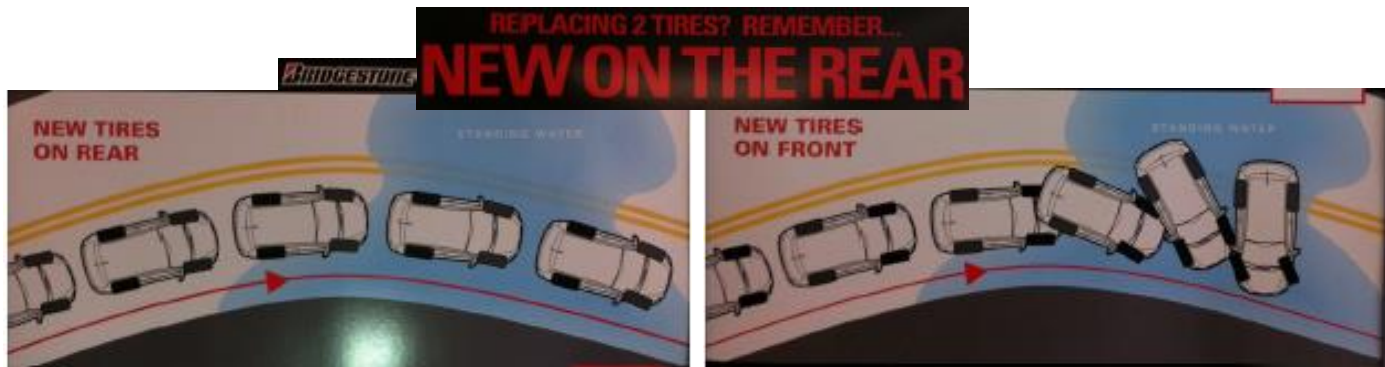
Fig. 3.48 Loss of directional stability due to lock-up of rear tires.
